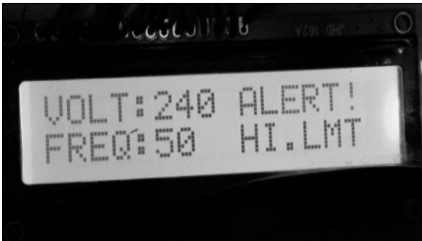
Fig 4: Alert shown for high voltage condition
