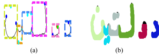
Figure 10: (a) the segmented characters borders on the thinned image of Fig.6. (b) The segmented characters.
