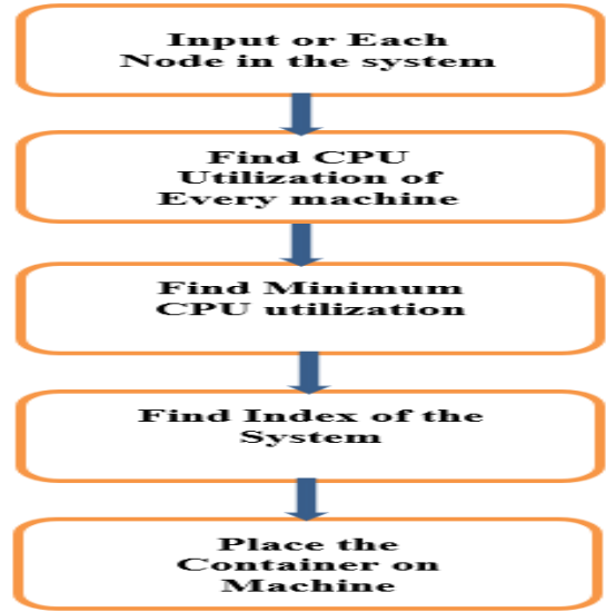
Fig.2. Process Flow of Optimizing Container Scheduling based Model
