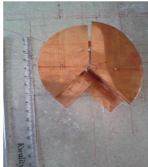
Fig 8: Fabricated prototype of gap-coupled shorted  $135^\circ$  S-MSAs
