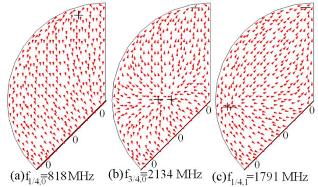
**Fig 2: Surface current distributions at various resonant modes for shorted 135° S-MSA for (a, b)  $x_f = 2.0$  and (c)  $x_f = 4.5$  [18]**
