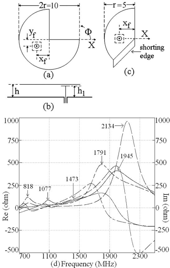
**Fig 1: (a) Top and (b) side views of 270° S-MSA, (c) shorted 135° S-MSA and (d) resonance curve plots for, (—) 270° S-MSA, shorted 135° S-MSA for (---)  $x_f = 2.0$  and (-.-)  $x_f = 4.5$  and  $y_f = 0$  [18]**
