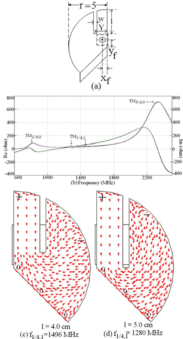
**Fig 3: (a) Slot cut shorted  $135^\circ$  S-MSA, its (b) resonance curve plots for  $l = (\text{---}) 0$ ,  $(\text{---}) 3$ ,  $(\text{---}) 4$ ,  $(\text{---}) 5$ , and its (c, d) surface current distribution at modified  $TM_{1/4,1}$  mode for two different slot lengths**
