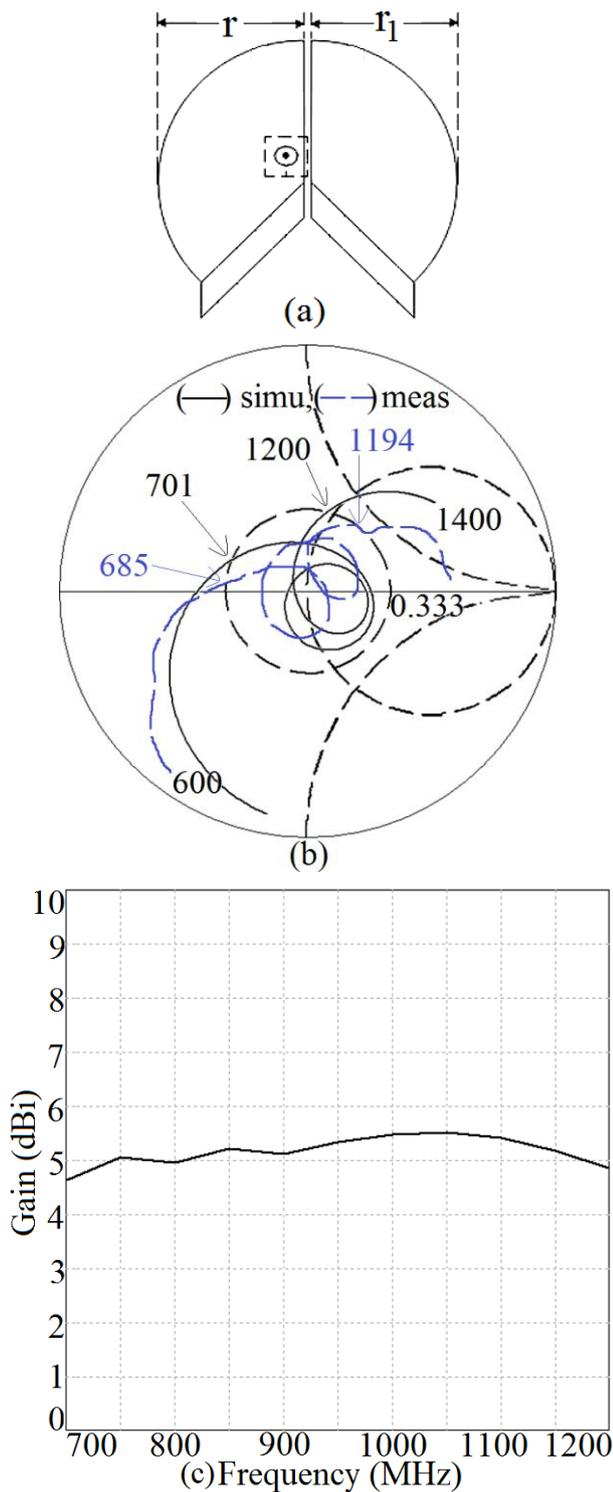
Fig 7: (a) Gap-coupled shorted  $135^\circ$  S-MSAs, its (b) input impedance plots and its (c) gain variation over the BW
