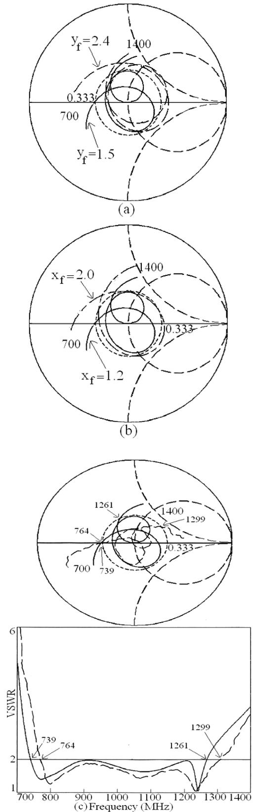
**Fig 4: Input impedance plots for (a)  $y_f = 2.4$ , (b)  $x_f = 2.0$ , and (c) optimized input impedance and VSWR plots for slot cut shorted  $135^\circ$  S-MSA,  $x_f = 1.2$ ,  $y_f = 1.5$**
