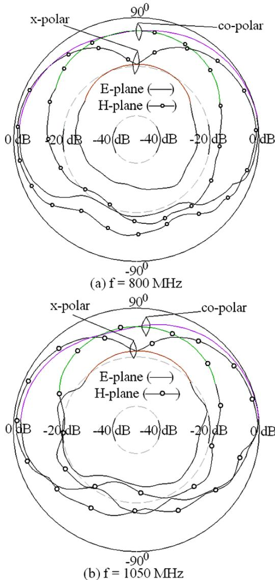
**Fig 5: (a, b) Radiation pattern plots at band start and center frequency of BW for slot cut shorted  $135^\circ$  S-MSA**
