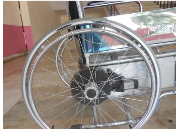
Fig 5.2 Geared assembly of the wheel
